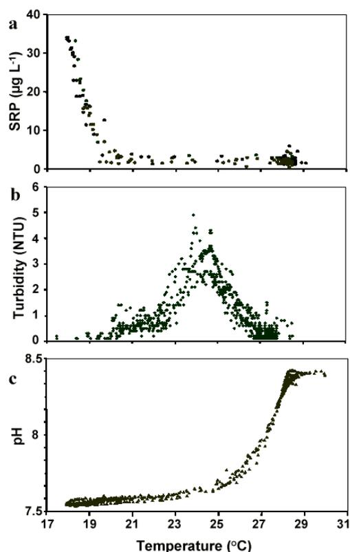
Fig. 4. Plot of (a) SRP, (b) turbidity, and (c) pH versus temperature from the datasets measured between July 8 and 9, 1999.
