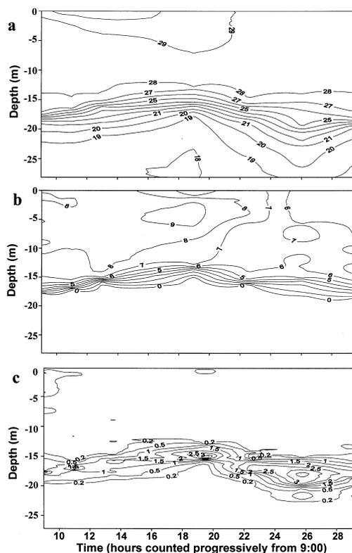
Fig. 2. Isopleth diagrams for (a) temperature ( $^{\circ}\text{C}$ ), (b) DO (ppm), and, (c) turbidity (NTU) drawn from profiles measured at the 28-m station between July 8 and 9, 1999.
