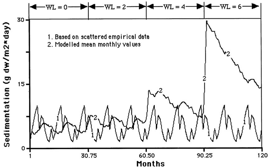
Fig. 8. A comparison between empirical data on sedimentation (Table 8) and model-predicted values for WL = 0, 2, 4 and 6 m. Note that the empirical data emanate from sediment traps sites for two water depths, and that the model predicts mean monthly values for A-areas.
