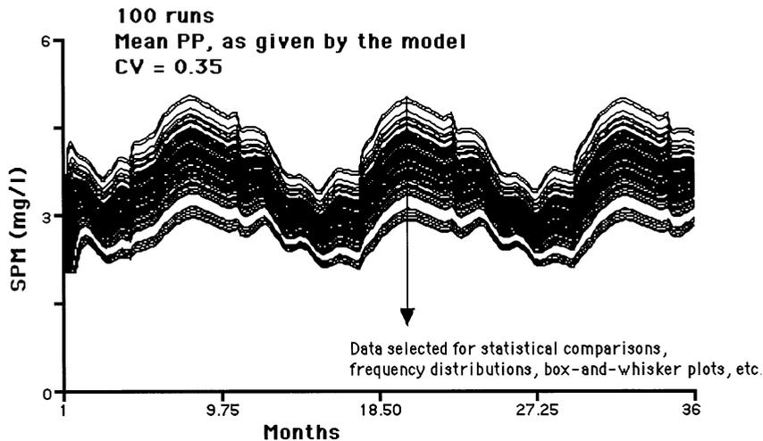
Fig. 11. Step one in the Monte Carlo simulations using the SPM-model (for  $WL = 0$ ). The target effect variable is SPM and the primary production (PP) has been varied ( $CV = 0.35$  and normal frequency distribution). One hundred runs. The figure also indicates that the following statistical analyses use data (MV, S.D. and  $CV = MV/S.D.$  for the month yielding highest SPM value).
