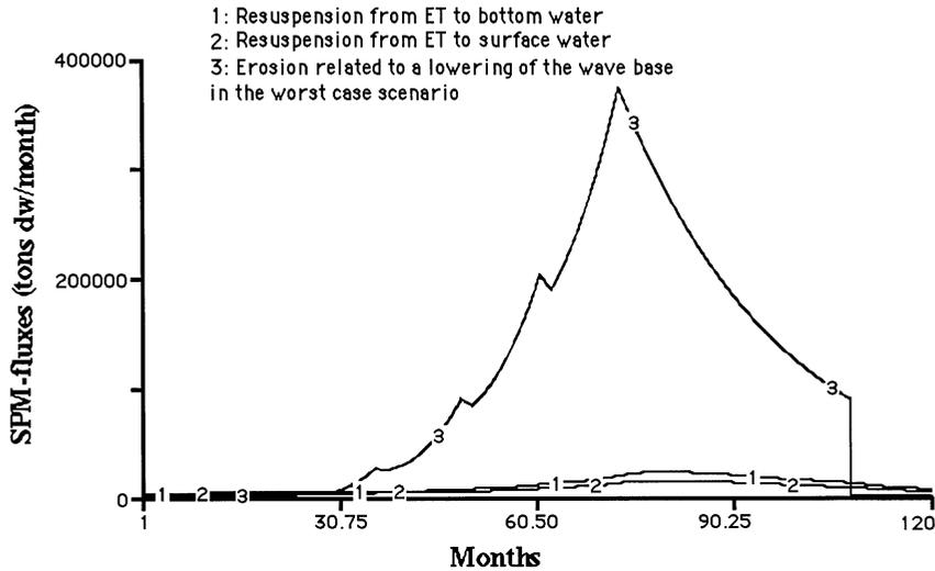
Fig. 15. Resuspension and erosion fluxes in the scenario with a gradual lowering of the water level.
