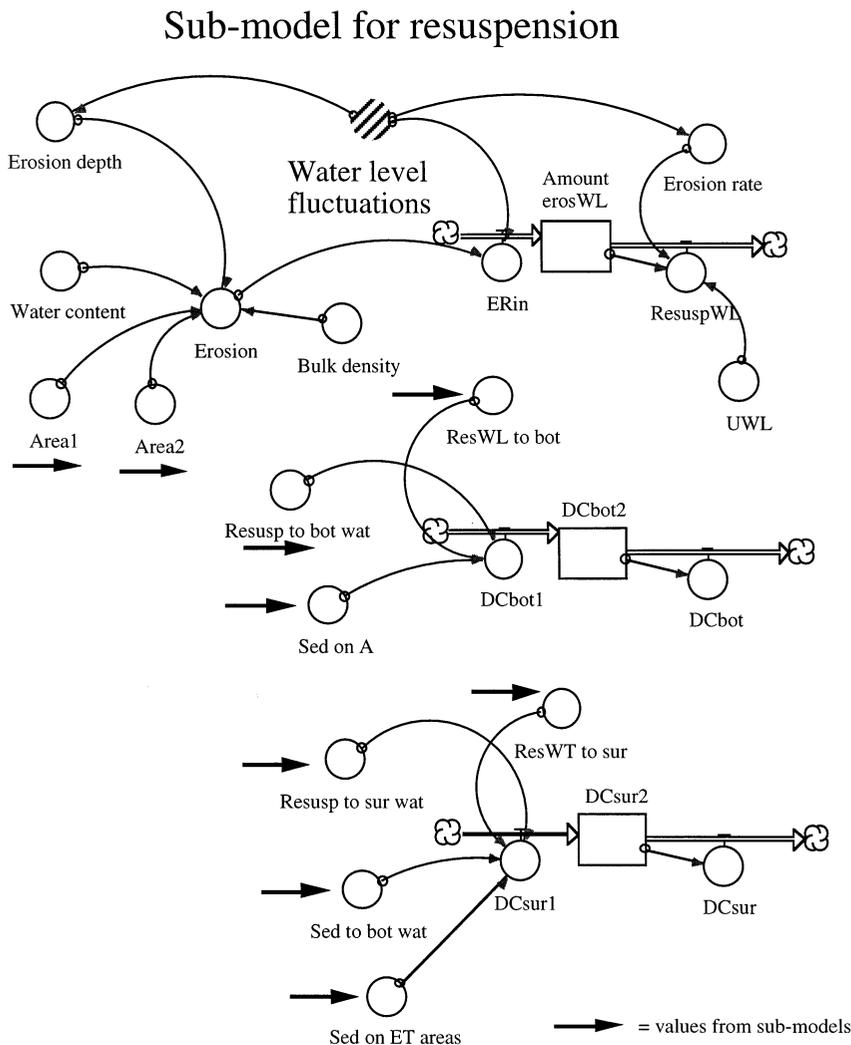
Fig. 7. An outline of the sub-model for resuspension and to calculate the distribution coefficient giving the fraction of resuspended matter relative to the total amount of suspended particulate matter in the water.
