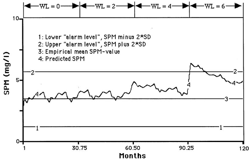
Fig. 9. A comparison between empirical data on SPM and model-predicted values for WL = 0, 2, 4 and 6 m. The lower and upper limits for 'alarm' are based on the mean empirical SPM-value (3.4 mg/l)  $\pm$  2 S.D. (S.D. = 1.13, corresponding to 95% confidence limits for individual values). Note that these are very wide limits when applied to the mean monthly SPM-values predicted by the model.
