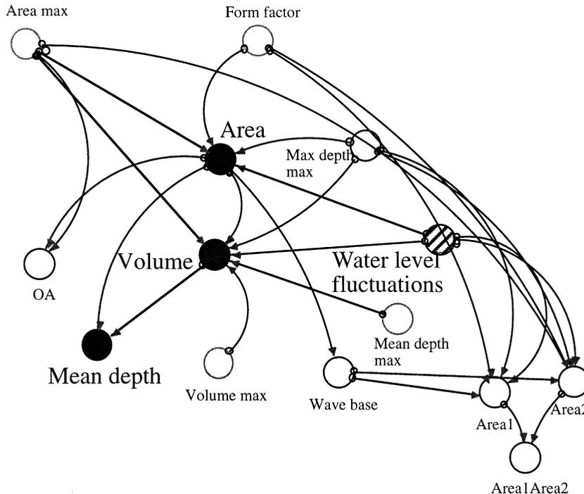
Fig. 5. An outline of the sub-model to calculate changes in lake area, volume and mean depth associated with water level fluctuations.
