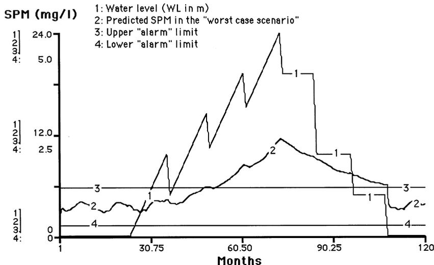
Fig. 14. Results for the scenario with a gradual lowering of the water level. The lower and upper limits for 'alarm' are based on the mean empirical SPM-value ( $3.4 \text{ mg/l} \pm 2 \text{ S.D.}$  ( $\text{S.D.} = 1.13$ , corresponding to 95% confidence limits for individual values). The driving function for these simulations is curve 1, the assumed changes in water level.
