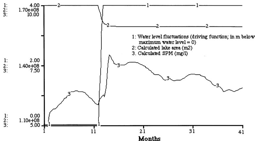
Fig. 13. Curve 1 gives the driving variable, water level fluctuations related to maximum area (WL = 0); curve 2 gives the calculated lake area related to the water level fluctuations; and curve 3 gives the target variable for these model calculations, the SPM-values.
