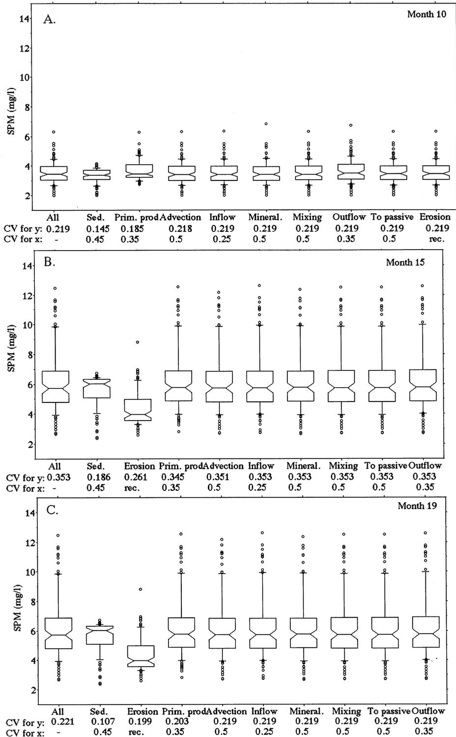
Fig. 12. Results of uncertainty analyses using the SPM-model for Lake Kinneret. All figures give calculated SPM-values on the y-axis, calculated CVs for the SPM-values as well as assumed CVs for the given processes. Upper: results for month 10, before changes in water level (the driving variable, see Fig. 13). Middle: results for month 15, 2 months after changes in water level (month 13). Lower: results for month 19.
