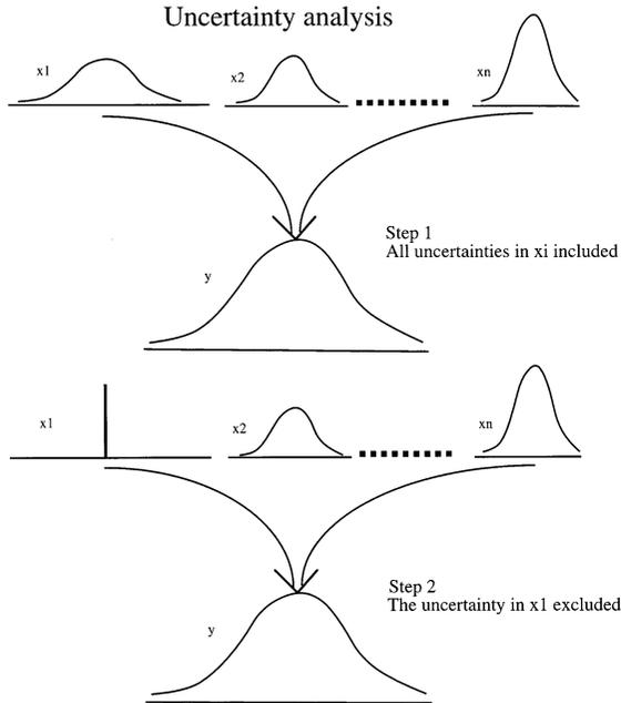
Fig. 10. Illustration of Monte Carlo simulations (= uncertainty analyses) as a two-step procedure (from Håkanson, 1999)
