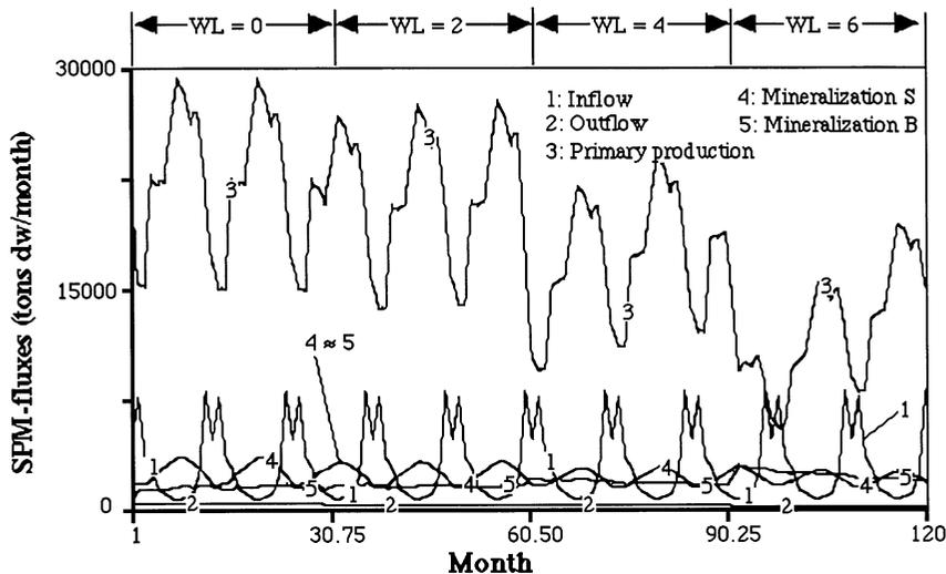
Fig. 3. Inflow, outflow, primary production, mineralization in surface water (S) and in bottom water (B) in Lake Kinneret, as predicted by the SPM-model for WL = 0, 2, 4, and 6 m.
